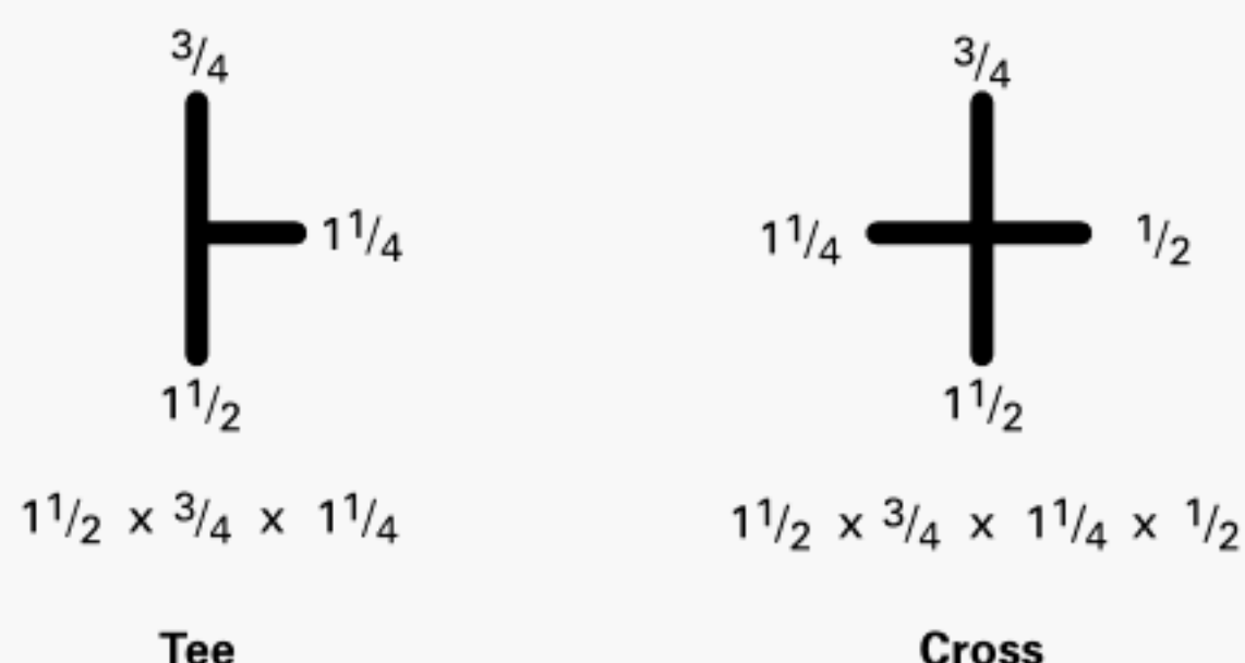
Figure 1 Method of Designating Outlets of Reducing Tees and Crosses
