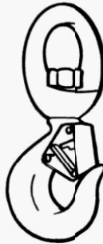
Fig. 10-1.1-11 Self-Closing Flapper Latch (Swivel Hook)
