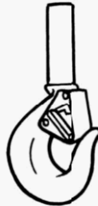
Fig. 10-1.1-10 Self-Closing Flapper Latch (Shank Hook)
