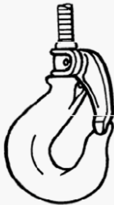
Fig. 10-1.1-9 Self-Closing Gate Latch (Shank Hook)
