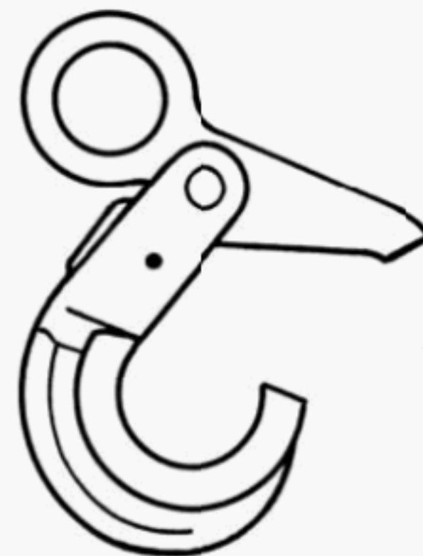
Fig. 10-1.1-6 Self-Locking Eye Hook (Open)
